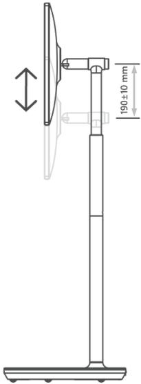
A side view of the TV on its stand. A vertical double-headed arrow indicates the height adjustment range. A dimension line to the right of the stand is labeled $190 \pm 10$ mm. |
